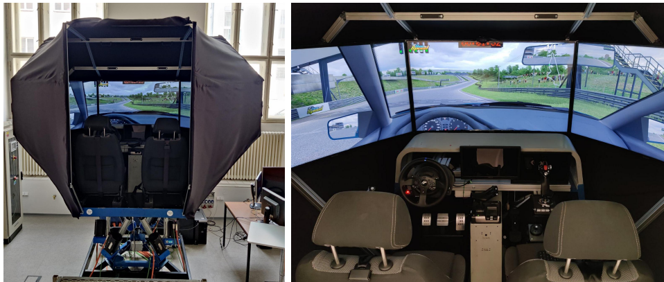
Figure 4.9: The 6-DoF motion platform used for the algorithm verification.
